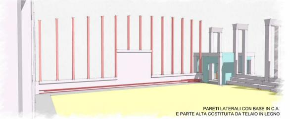
PARETI LATERALI CON BASE IN C.A. E PARTE ALTA COSTITUITA DA TELAIO IN LEGNO
